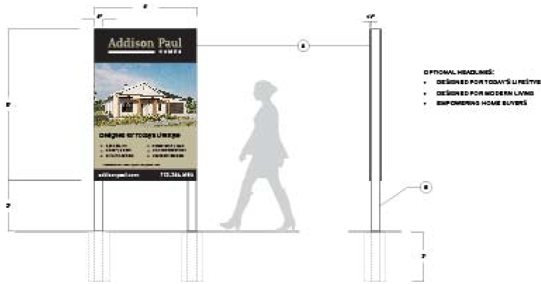
CONSTRUCTION SIGN OPT A SCALE: 1/2"=1'-0"
