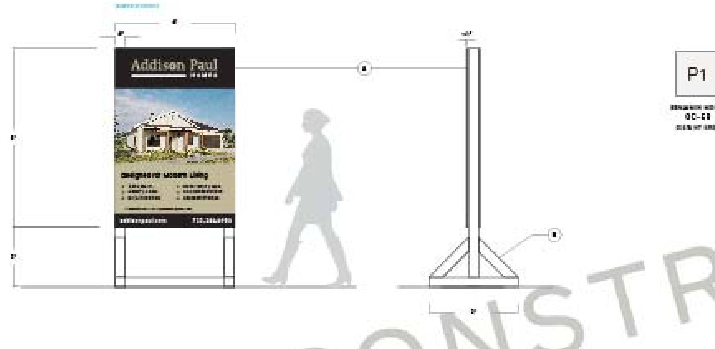
CONSTRUCTION SIGN OPT B SCALE: 1/2"=1'-0"
